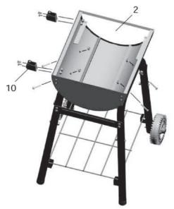
6. Place in straight pisizone, the base of the carriage thus assembled. Attach the chamber combustion (2) to the trolley using 4 1/4-20x1-3/4" hex bolts and nuts 1/4-20. Note: Make sure the ash tray opening is positioned on the same side as the wheels.
