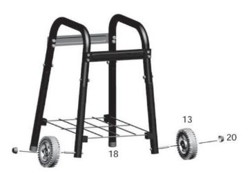
5. Insert the wheels (13) to the axle, then close with the wheel covers. Then insert the feet (18) to the end of the long legs.
