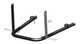
2. Insert the two leg supports (21) outside the assembled legs, using 4 1/4-20x1-3/4" hex bolts and 1/4-20 nuts
