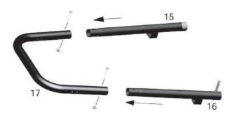
1. Insert the base of the long legs (15) and the base of the short legs (16) to the upper part of the legs (17) and screw in with 2 hexagonal bolts 1/4-20x1-3/4" and the 1/4-20 nuts. Repeat this step for the other legs
