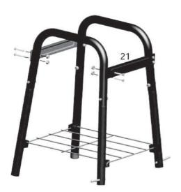
4. Assemble the other end of the leg supports (21) to the corresponding leg using the  $4\ 1/4-20x1-3/4$ " hex bolts and 1/4-20 nuts.
